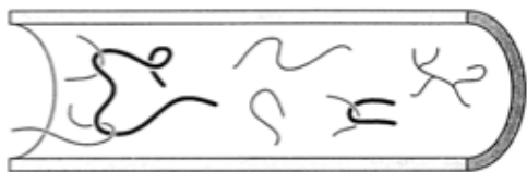
Figure 3 Collisions between long DNA molecules and the polymer chains of solution provide very fast separations.
